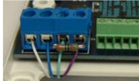
Termination of NOX bus with a 120–180Ω ¼ W resistor between bus legs A og B.
